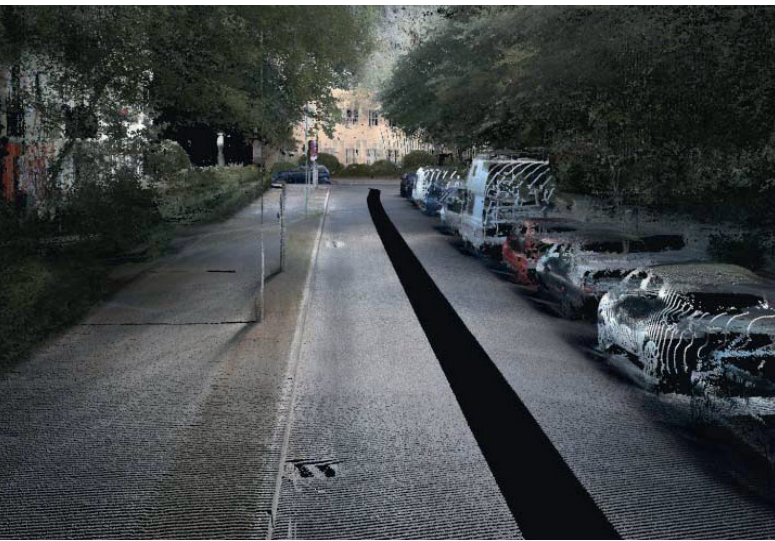
Left: Textured point cloud, reconstructed from data taken at 50 km/h with a CPS laser scanner and four cameras. Right: Automatically segmented point cloud. Data interpretation was realized by using an automated 3D data interpretation software 3D-AI developed by Fraunhofer IPM.
